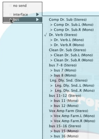
Figure 4-37: Use the Sends window to pick where to send your track's signal for effects processing.
